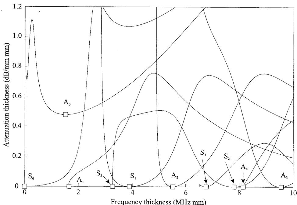
**Figure 5.** Attenuation curves for a steel plate in water. The squares indicate local minima in the attenuation for each mode.
