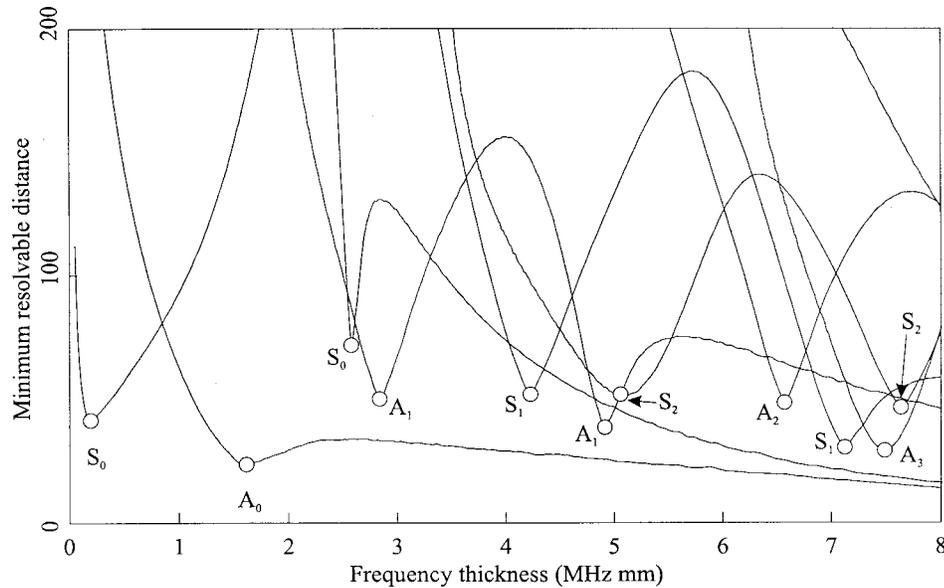
Figure 4. MRD curves for a steel plate and a propagation distance to plate thickness ratio of 800. The circles indicate local minima in the MRD for each mode.
