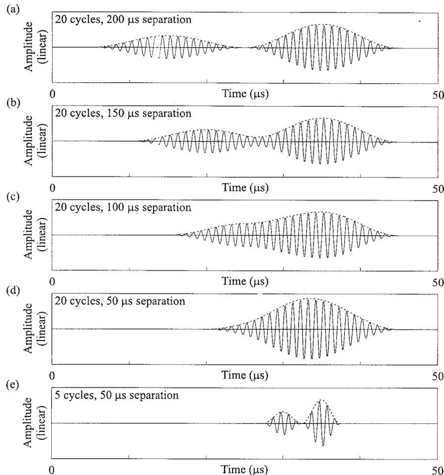
**Figure 3.** Predicted time-traces showing (a) two twenty-cycle wave-packets with centre frequencies of 1 MHz completely separated in time. The effect of progressively reducing the separation between centres of the wave-packets is illustrated in time-traces (b), (c) and (d). Time-trace (e) shows the effect of reducing the number of cycles in the wave-packet to five while maintaining the same separation between the centres of the wave-packets as in time-trace (d).
