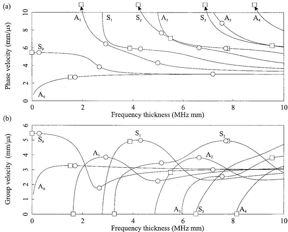
**Figure 1.** (a) Phase and (b) group velocity dispersion curves for a steel plate in vacuum. Circles indicate local minima in minimum resolvable distance (MRD) and squares indicate local minima in attenuation for the same plate immersed in water.
