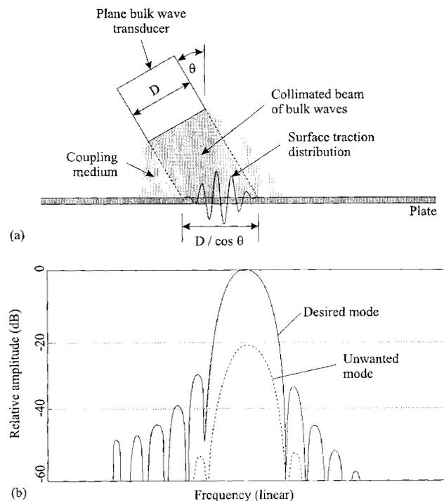
**Figure 6.** (a) Schematic diagram showing an angle incidence transduction configuration when used as a transmitter and (b) a typical modal selectivity plot.
