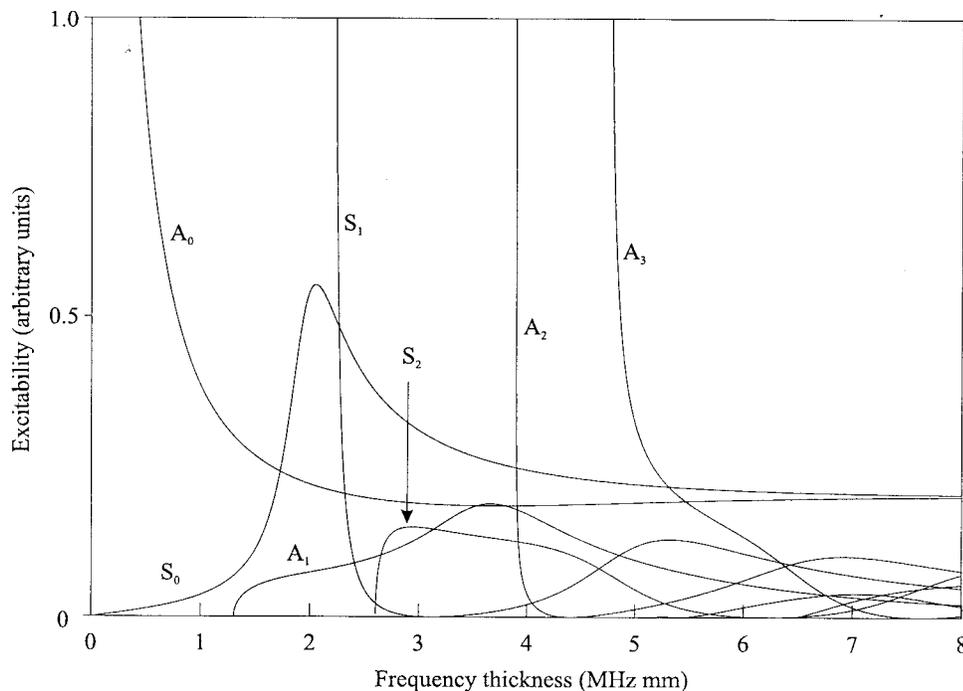
Figure 7. Out-of-plane excitability curves for a steel plate.
