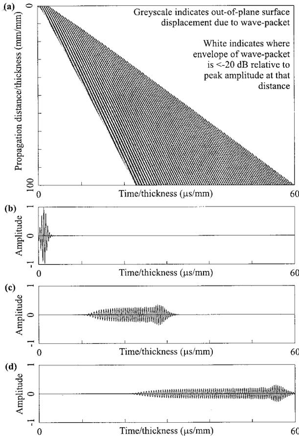
**Figure 2.** An example of dispersive wave propagation. (a) Shows a numerical prediction of the spreading of the  $S_0$  mode in a steel plate when the input signal is a five-cycle Hanning windowed toneburst with a centre  $f_d$  at 2.0 MHz mm. On the right hand side are numerical predictions of three time traces that would be received at propagation distance to thickness ratios of (b) 0.1, (c) 50 and (d) 100.
