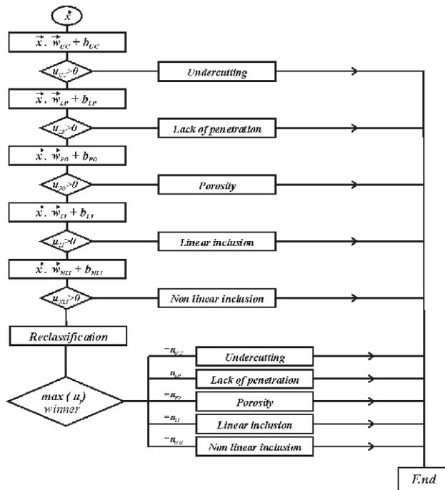
**Figure 5. Algorithm of the non-hierarchical classifier**
