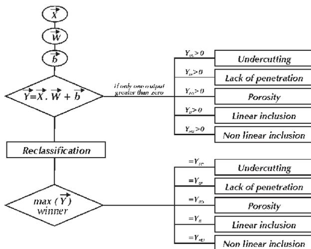
**Figure 6. Algorithm of the hierarchical classifier**
