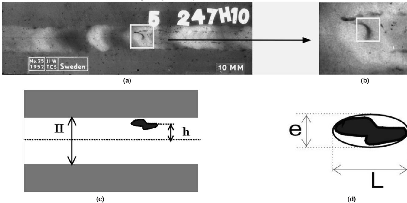
Figure 2. (a) Example of pattern IIW used; (b) presence of slag inclusion; (c) and (d) illustration for definition of the parameters used
