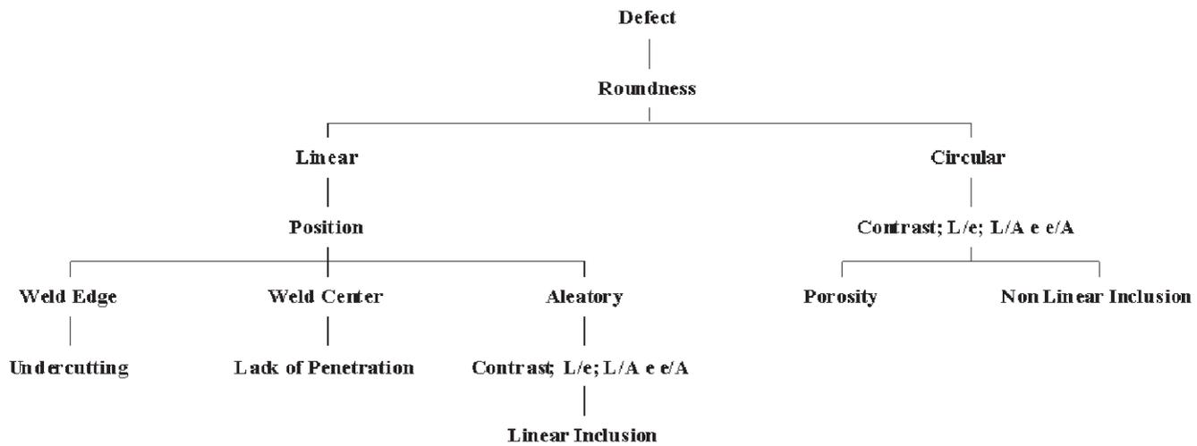
Figure 1. Chart representing the separation of the classes of defects through the used parameters
