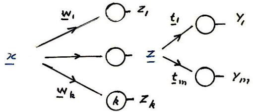
$$\Delta w_{ij} = -\alpha \frac{\partial F}{\partial w_{ij}} = -\alpha \sum_l \frac{\partial F}{\partial \tilde{y}_l} \frac{\partial \tilde{y}_l}{\partial u_l} \frac{\partial u_l}{\partial z_i} \frac{\partial z_i}{\partial v_i} \frac{\partial v_i}{\partial w_i}$$
