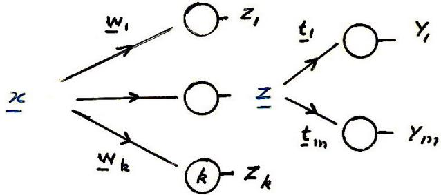
$$\tilde{y}_l = \tanh(u_l) \quad u_l = \sum_i t_{li} z_i \quad z_i = \beta v_i + \tanh(v_i) \quad v_i = \sum_i w_{ij} x_i$$
