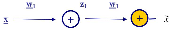
$$\tilde{x} = z_1 \underline{w}_1 = \underline{w}_1^t \underline{x} \underline{w}_1$$
