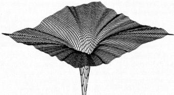
Fig. 23. Example MSE surface of sigmoid error.
