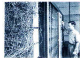
Fig. 1.B. • The Mark I Perceptron patchboard. The connections between the perceptron and the computer were typically 'random', so as to discover the ability of the perceptron to learn the desired pattern without need for pre-programming. Photo courtesy of Aeron Calapan Advanced Technology Center.
